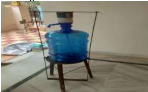
Fig.1. Reciprocating Leg Operated Washing hands Dispenser Fig.2. Drinking Water System
