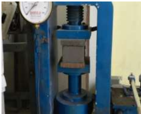
Figure 9: Testing of 10%MSW specimen at 7 days curing
