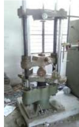
Figure 10: Split tensile strength testing at 5% Plastic at 14 days curing
