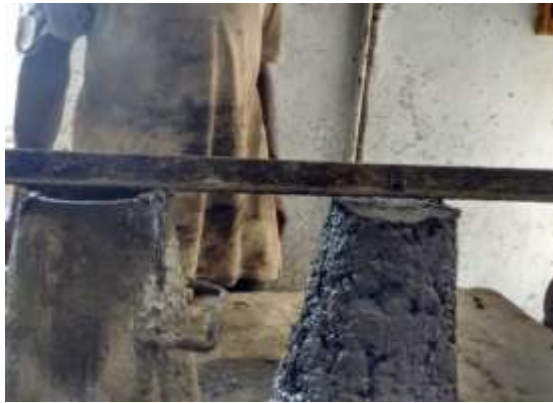
Slump cone test
