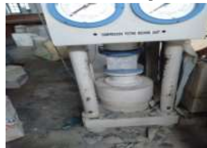
Cube compressive strength test
