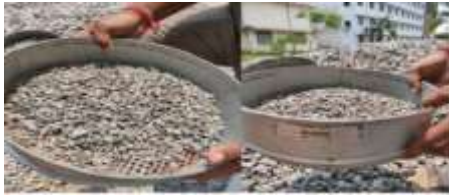
Fig 4: 20mm coarse aggregates and 12mm coarse aggregates
