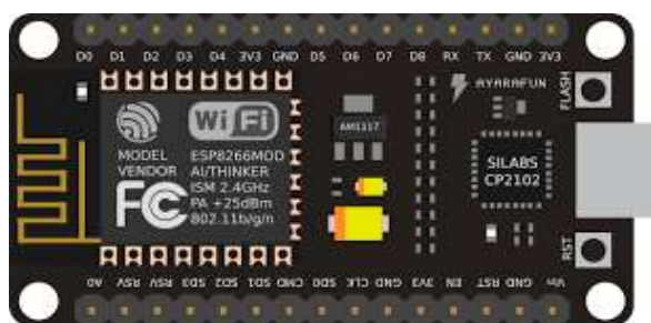
Fig 2 - Node Microcontroller ESP8266
