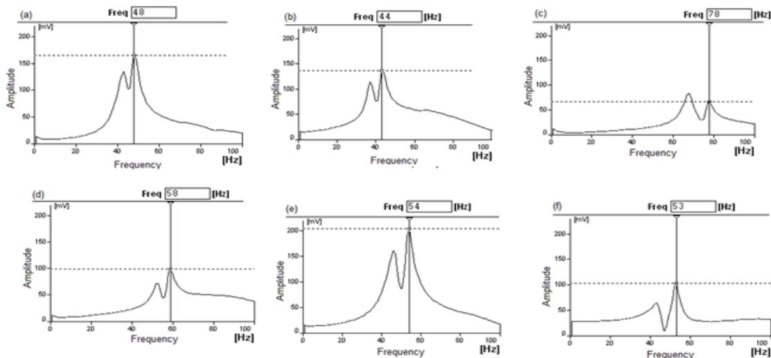
Figure 3. Frequency responses of neutralizer by experimental modal analysis when neutralizer is tuned to impose node at, (a) 1L, (b) 0.9L, (c) 0.7L, (d) 0.6L, (e) 0.5L, and (f) 0.4L for  $\omega_e = 22\sqrt{EI/(\rho L^4)}$ .
