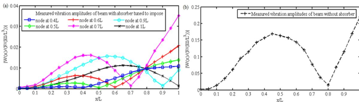
Figure 2 Experimental measured vibration amplitudes of a uniform cantilever beam, (a) with, neutralizer tuned to the resonance frequency to create node at different locations and (b) without neutralizer. The experimental parameters are  $\omega_e = 53\text{HZ} \approx 22\sqrt{EI/(\rho L^4)}$ ,  $x_f = 1000\text{mm}=1L$ ,  $x_p = 400\text{mm} = 0.4L$ , and  $m_1 = 0.5\text{kg} = 0.1\rho L$ .
