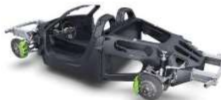
Figure 1.4 Porsche 918 Spyder CFRP monocoque chassis
