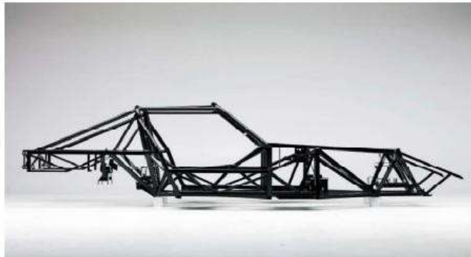
Figure 1.1 Space frame chassis
