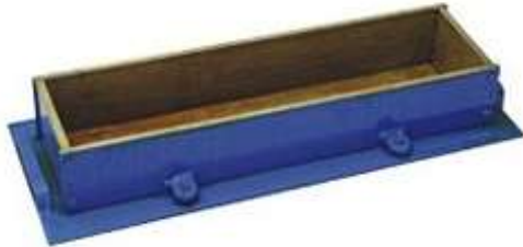
Fig 3. 7 150 x 150 x 700 mm prism
