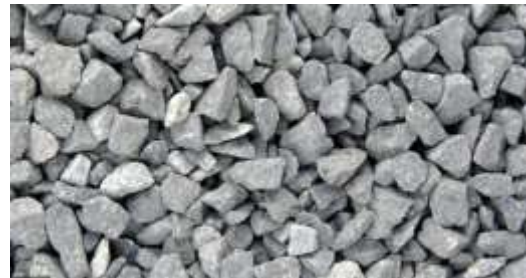
Fig 3. 2 coarse aggregates of 20 mm
