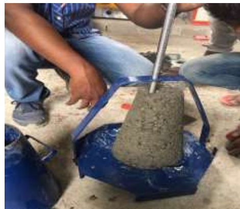
Fig 4. 1 Test of cone slump
