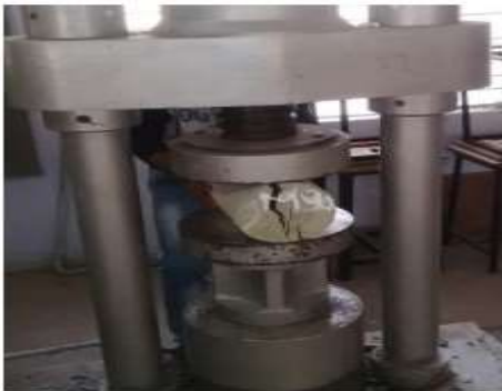
Fig 4. 4 Testing for Split Tensile Strength
