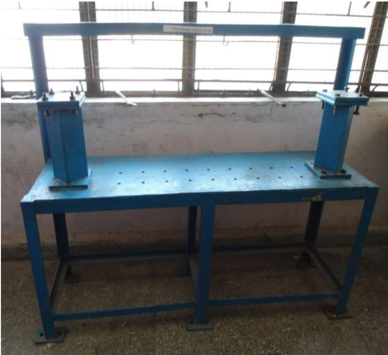
Figure 2: Actual experimental set-up for vibration analysis and crack detection
