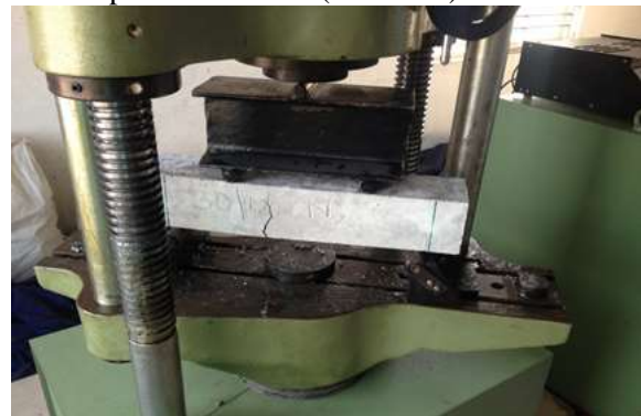
TESTING OF FLEXURAL STRENGTH IN UTM
