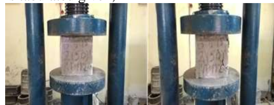
Fig.4.4.1 Compressive Strength Test of Cubes
