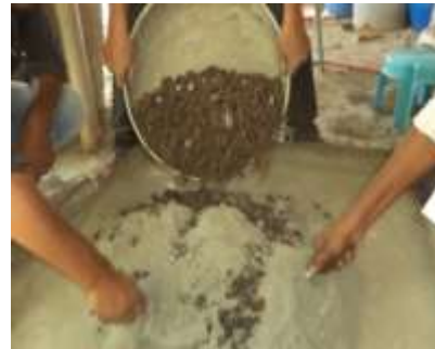
Plate 4.10 Mixing of cinder with cement
