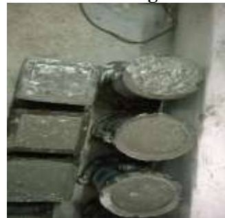
Plate 4.13 Casted cubes and cylinders
