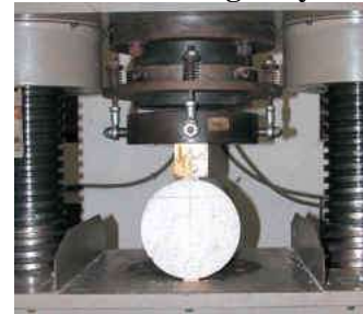
Plate 4.5 Testing of cylinder by split tensile
