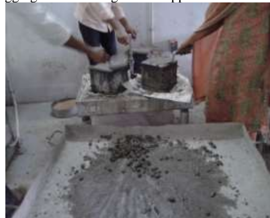
Plate 4.1 Casting of cubes with vibrator 4.2.9 Curing procedure
