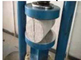
Plate 4.15 Crack pattern of cylinder
