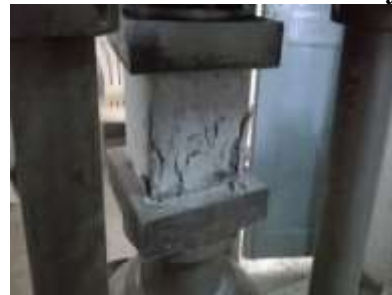
Plate 4.14 Crack pattern of cube
