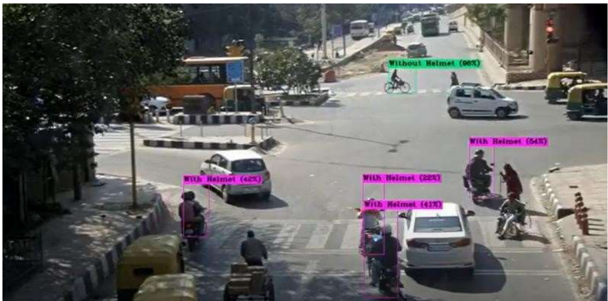
Fig 2: Helmet detection snapshot from video using YoloV5
