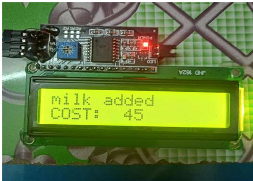
Fig3 - When a product is added in basket it displays the confirmation in LCD
