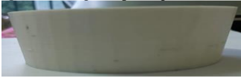
Fig. 8 (a) PLA plunger cup front view
