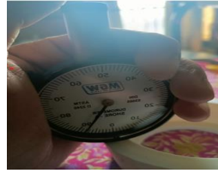
Fig. 2. Durometer test of cup
