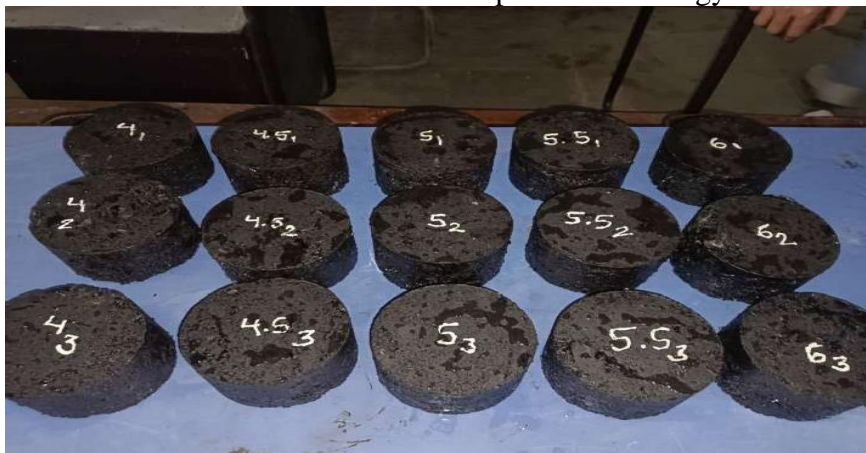
Fig. 2 : Samples with varying bitumen content
