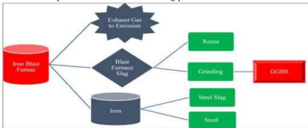
Figure 1.3 - Manufacturing Process of GGBS
