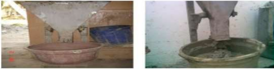
Figure.2. Funnel test apparatus (SSC Mixes)
