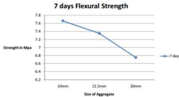
Figure.16: 7 days Flexural strength with various sizes of Aggregates
