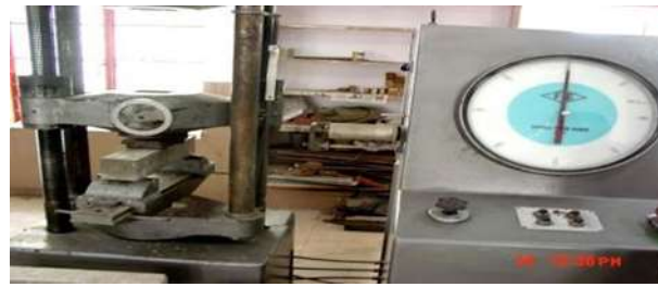
Figure .5. Flexural strength test
