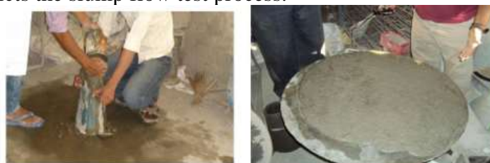
Figure.1. Slump flow test and T50 cm test procedure (SCC mixes)
