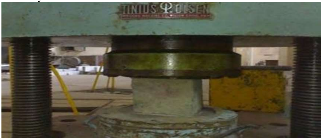
Figure.4. Compressive strength test setup
