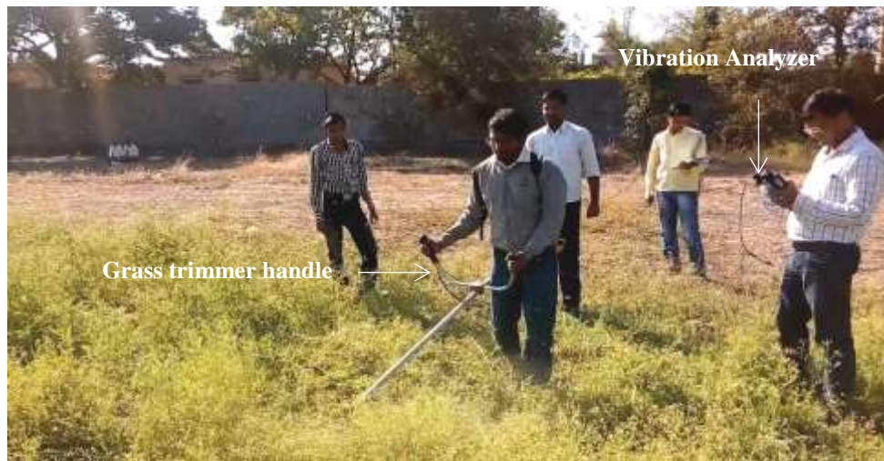
Figure 4: Frequency spectrum measurement of trimmer during cutting operation.
