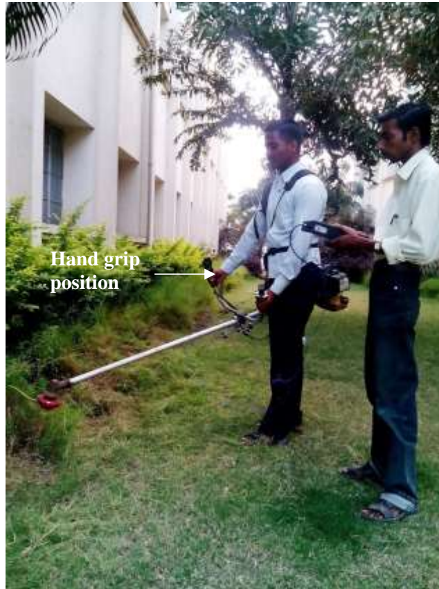
Figure 8: Handle vibration measurement during cutting operation.
