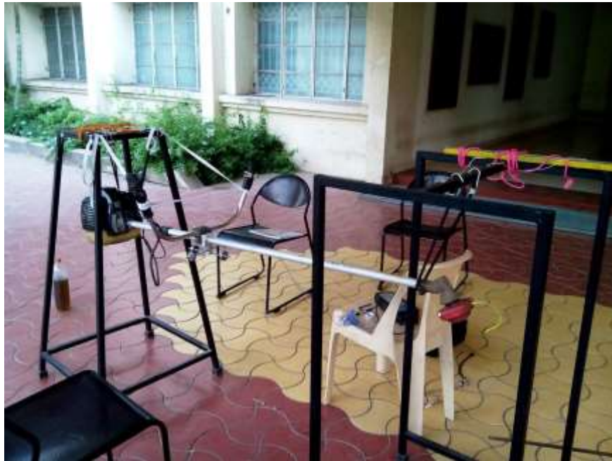
Figure 6: Grass trimmer setup for vibration measurements along pipe.
