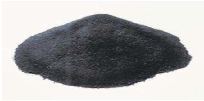
Figure 1 Treated pulverized waste foundry sand The Physical properties of TPWFS are noted in Table 1.
