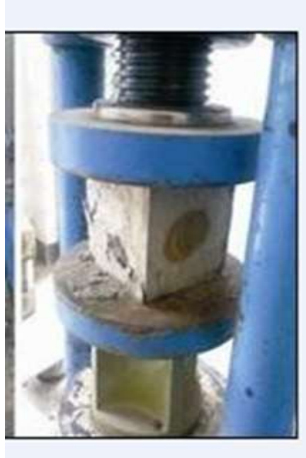
Figure.5.1 Compression Strength Testing Machine
