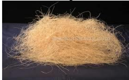
Figure 2: Image of coconut coir used as reinforcement
