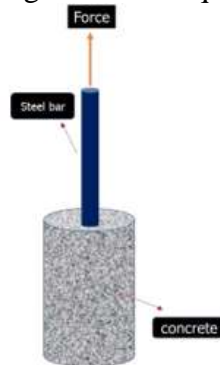
Fig.4. Typical bond between concrete and steel
