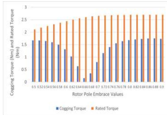
Fig. 6 Cogging Torque and Rated Torque vs Pole Embrace Factor
