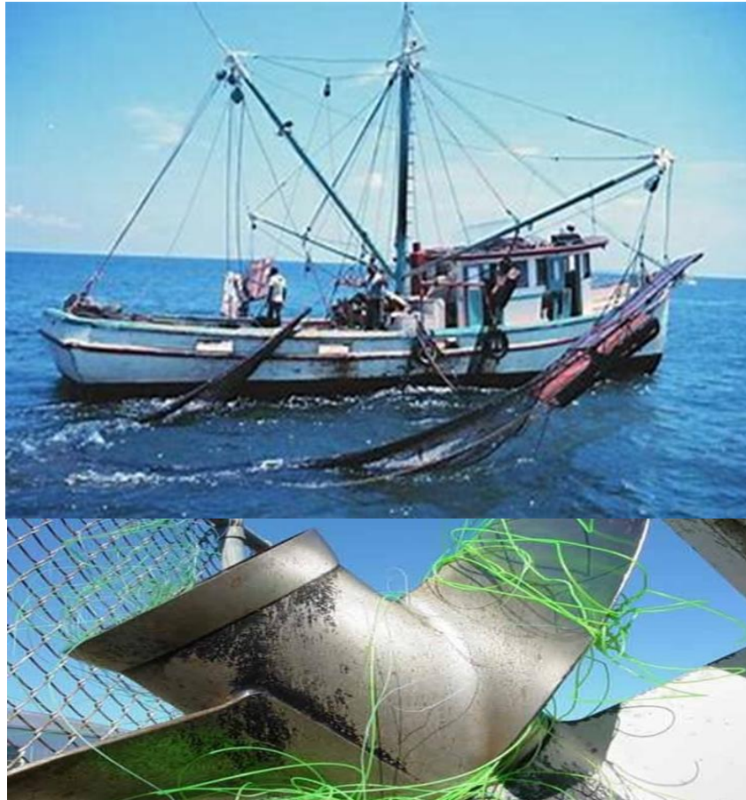
Damaged net due to jamming in propeller
