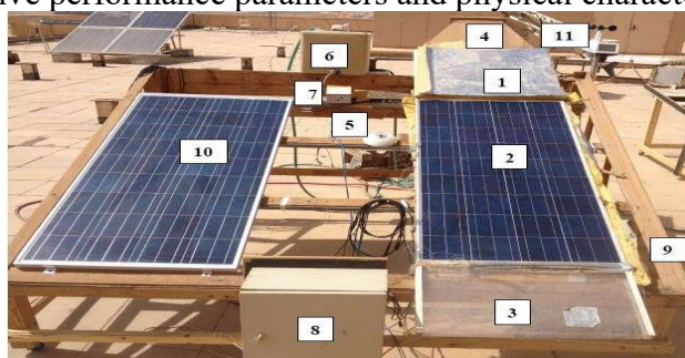
“Fig 3: Experiment set up: 1: entrance section, 2: PV panel with cooling, 3: exit section, 4: fan (20W) assembly, 5: pyranometer, 6: water tank, 7: water flow meter, 8: electrical connection box, 9: wooden pool with 24° inclination facing south, 10: reference panel and 11: weather station.”
