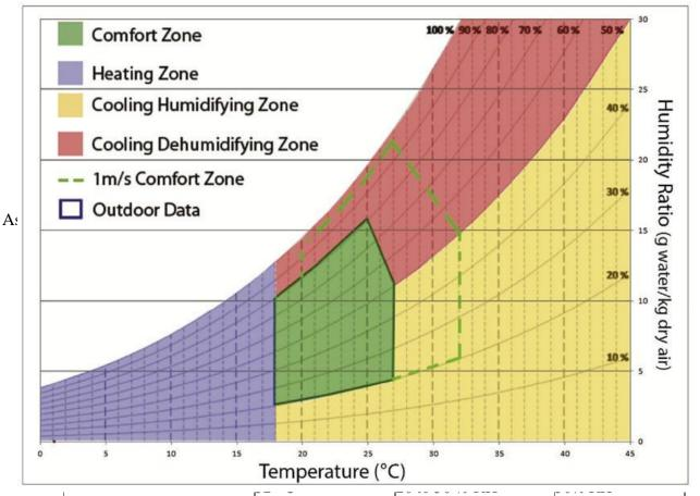
Considering the above parameters for human comfort Zone, the supply air temperature and humidity range is defined.
