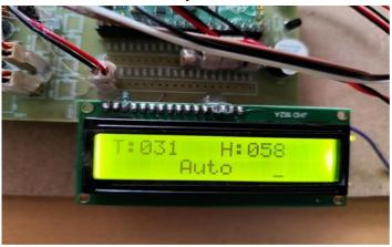
The LED displays the Temperature and humidity levels and mode switches on LED by sensing the grain humidity values. We can see in the above placed picture how the values are represented.
