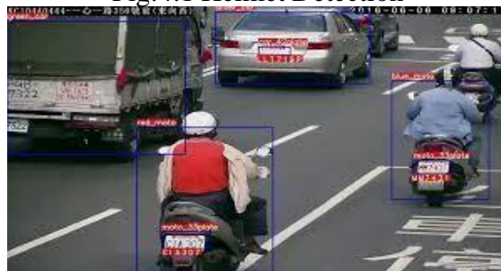
Fig:4.2 Detecting multiple Vehicles
