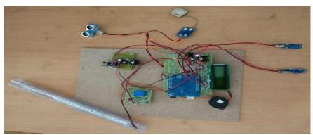
The above image shows the hardware equipment of the project. The kit is turned ON by giving the regulated power supply of 12v which is then converted to 5v dc current. The generated 5v dc current passes to every hardware component in the circuit.
