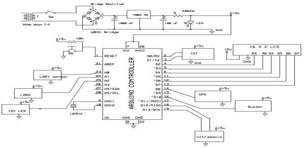
This is the pin diagram where all the hardware components are been connected components. this ARDUINO microcontroller having 28 pins. In which 14 GPIO pins as digital pins and 6 GPIO pins. 16MHz crystal oscillator connected internally. The step down transformer, Bridge rectifier capacitor with 1000f Resisters and led are connected in Regulated power supply which provide the 5v to the Arduino and all input/output modules.
