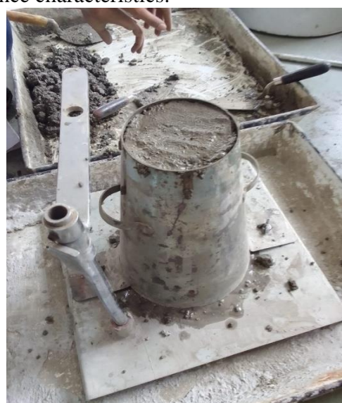
Fig.2. Slump cone mould
