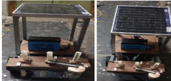
Figure 10: final Solar Powered Seed Sowing Machine
