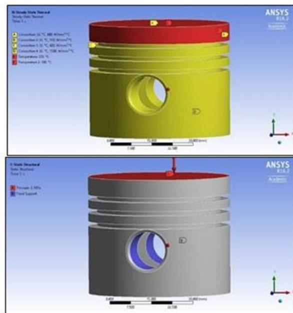
Figure 7, Steady state thermal boundary conditions for piston
