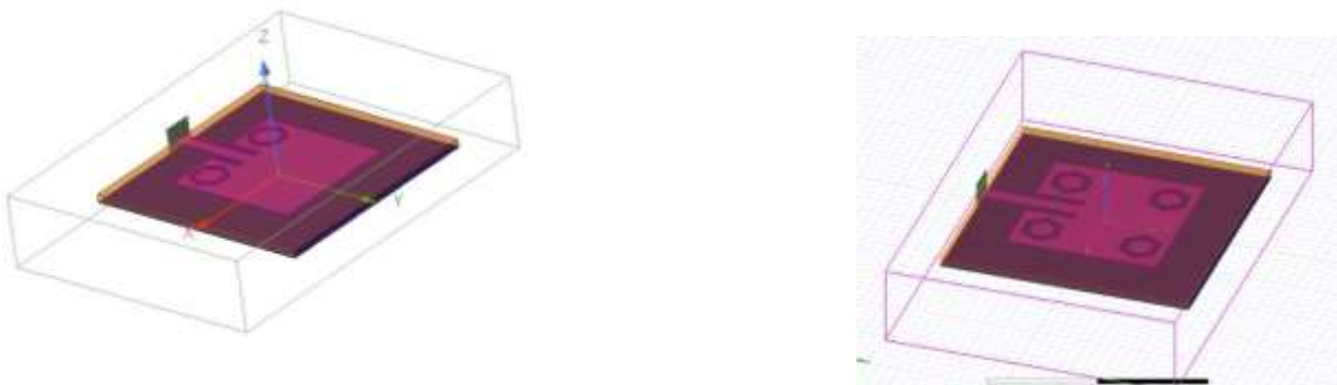
Figure 7: Metamaterial inspired square patch antenna (a) 2 hexagons (b) 4 hexagons shape.
