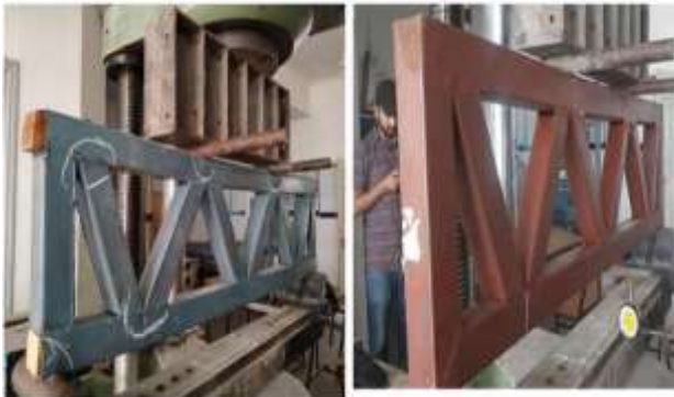
Figure No 3: Failure of Cold Form Steel and Hot Rolled Steel
