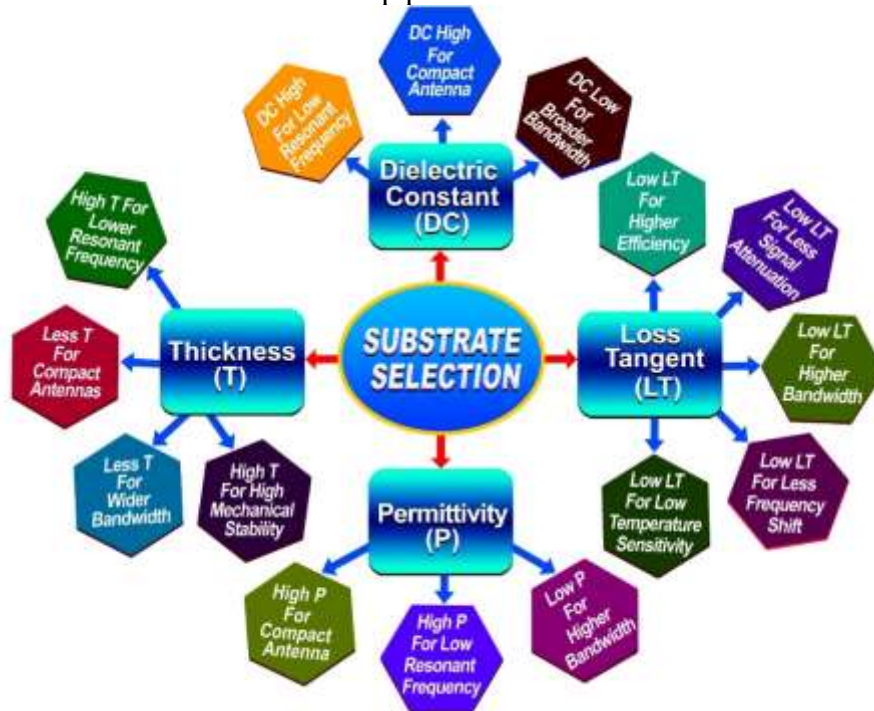
Fig 2. Characteristics for the selection of substrate in Wearable Antennas
