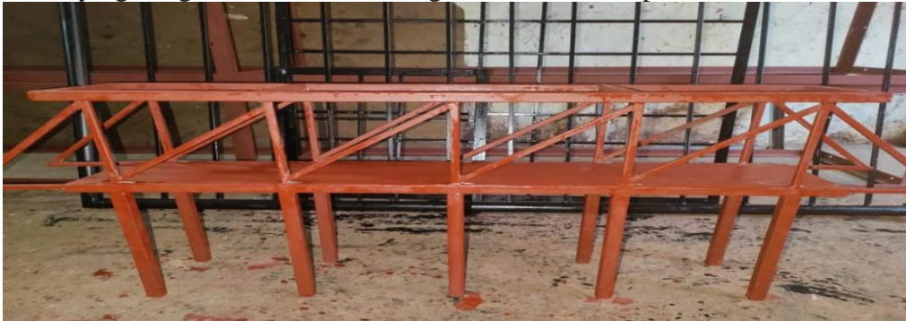
Fig 4.1 Steel Bridge Model
