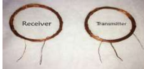
Fig.2: Transmitting & Receiving coils
