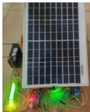
Fig – Hardware model of the cooling system with air cooling and orientation tracking using Arduino
