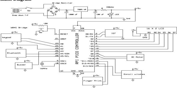
This is the pin diagram where all the hardware components are been connected components. this RPI PICO microcontroller having 28 pins. In which 14 GPIO pins as digital pins and 6 GPIO pins. 16MHz crystal oscillator connected internally. The step down transformer, Bridge rectifier capacitor with 1000f Resisters and led are connected in Regulated power supply which provide the 5v to the Arduino and all input/output modules.
