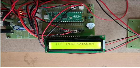
When we hit the reset button after providing the regulated power supply, the LCD displayed the IOT PDA System. The output is seen in the following image after we have connected the IOT module via a WIFI connect and after completing all the security verifications.
