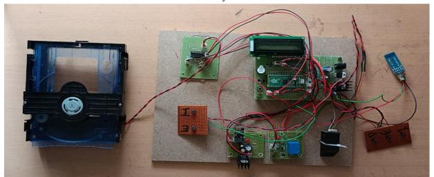
The above image shows the hardware equipment of the project. The kit is turned ON by giving the regulated power supply of 12v which is then converted to 5v dc current. The LED is the indication for 5v current so, if there is 5v current then automatically the LED glows. The generated 5v dc
