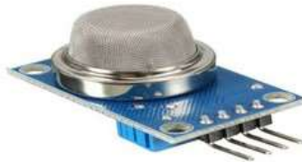
Fig. 4.5 Air Quality Sensor
