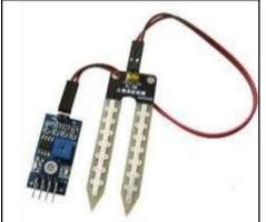
A soil humidity detector is a detector that senses the moisture content of the soil. The sensor has both analogue and virtual affairs. The virtual affair is constant, and the analogue output threshold may be
