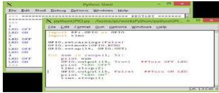
Fig. 17: GPIO LED Output
