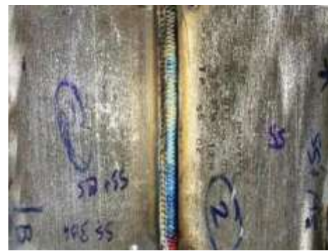
Figure.6 Stainless steel material with weld joint of Stainless steel
