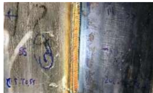
Figure.7 Carbon steel material with weld joint of Stainless steel
