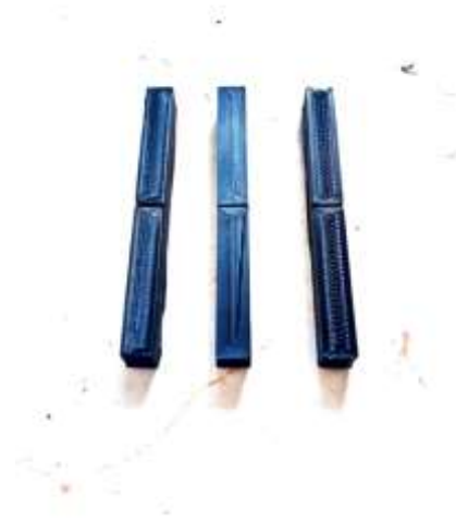
Figure 3.1 Printed Impact Specimens
