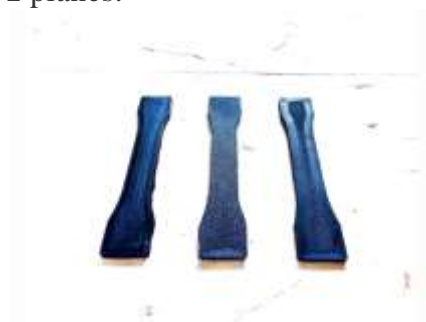
Figure 3.4 Printed Tensile Specimens
