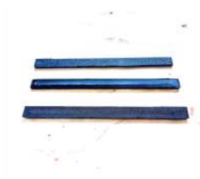
Figure 3.3 Printed Flexural Specimens
