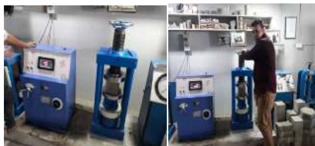
Fig. 3 Testing of cubes
