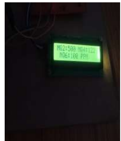
Fig .4.2 : Different gases ppm display on the LCD display
