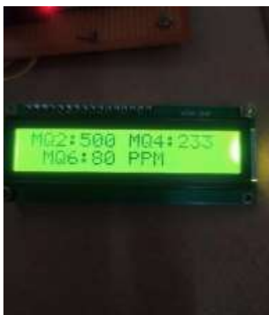
Fig .4.2 : Different gases ppm display on the LCD display
