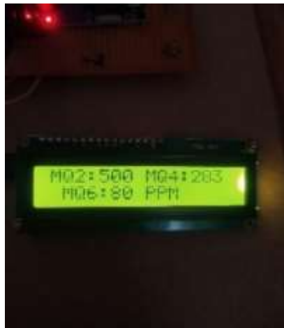
Fig .4.2 : Different gases ppm display on the LCD display
