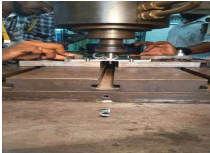
Fig:6 BTFSW Welding Operation
