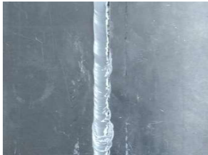
Fig:7 BTFSW WeldedSpecimen
