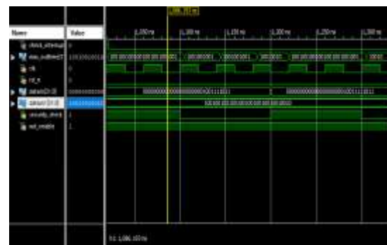
Figure 4: Simulation of Proposed Watchdog Timer
