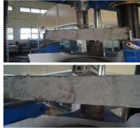
Fig.11 Flexural Strength tests of beam samples in UTM
