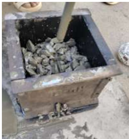
Fig.7 casting of cube
