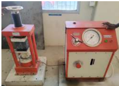
Fig.10 testing of cube specimen
