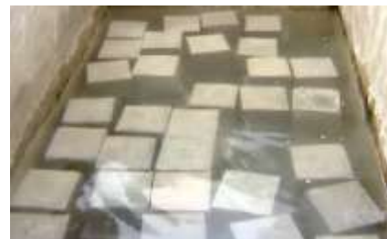
Fig.9 Specimens in Curing Tank
