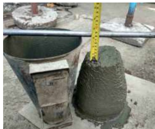
Fig.6 Slump cone test
